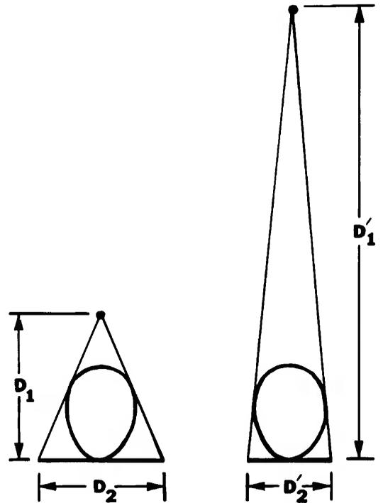
FIGURE 37.—Variation in parallax distortion ( $D_2$ ) of X-ray images due to differences in focal spot to film plane distances ( $D_1$ ).
